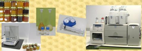
Standard solutions of glucose, fructose and sucrose, were used to identify and quantify the individual sugar components in the honey samples
