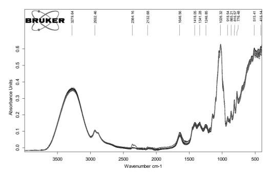
Figure 2 - FTIR- ATR spectrum of the average spectra from honeys acquired from 4000 to 450 cm<sup>-1</sup>.
